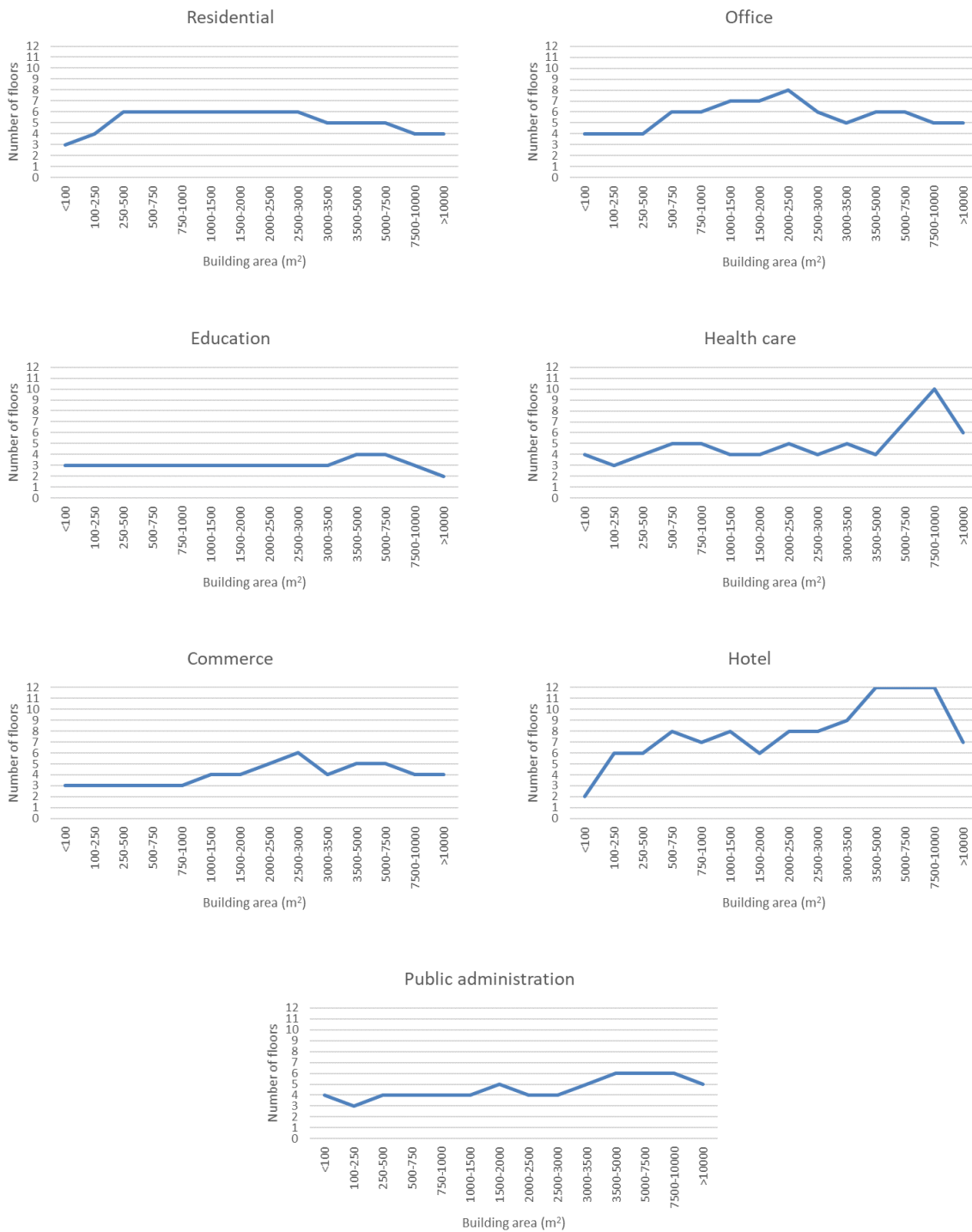
Figure 23 - Building height-area analysis that is integrated in the tool for energy demand calculation
